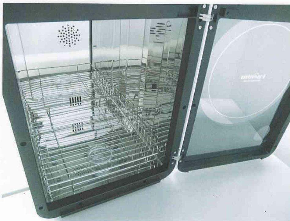
Photo 2. Example of position of test specimen: Lower row
